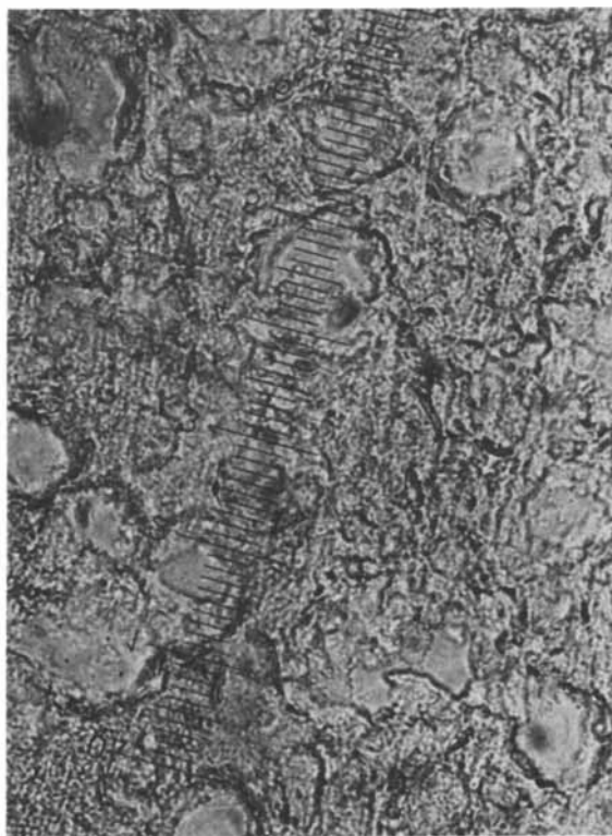
Figure 1. Structure of W/O emulsion containing microcrystalline wax as revealed by polarization microscopy (950 \times )
